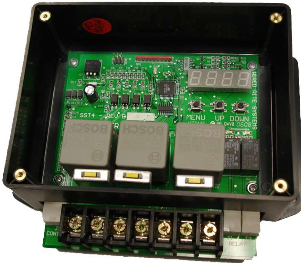
Figure 1. SST-4 in enclosure with cover removed
