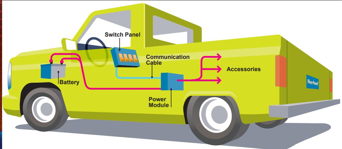
Flex-Panel may be used for any vehicle electrical power distribution and control application, including work trucks, utility vehicles, emergency, fire and police vehicles. A generic simplified system installation is shown above. The Flex-Panel Control System can be customized for each specific vehicle application.
